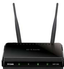
Gambar 3.3. Contoh access point Indoor.
